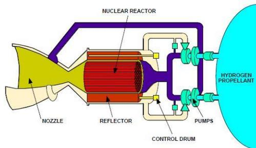
**Fig. 1.** Major elements of a nuclear thermal propulsion system<sup>1</sup>.
