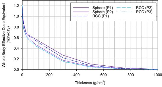
Fig. 3: Whole Body Effective Dose Equivalent as a function of Thickness of Polyethylene
