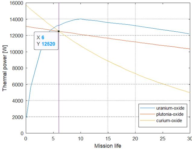
**Fig. 3.** Plutonium, uranium and curium based ceramic fuels are compared. The graph shows thermal power as a function of time.
