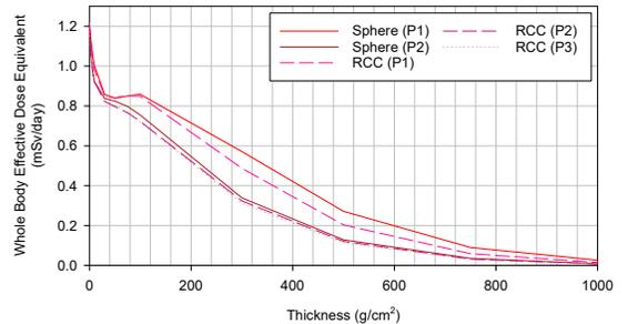
Fig. 5: Whole Body Effective Dose Equivalent as a function of Aluminum Thickness
