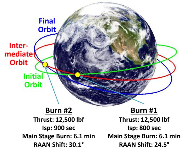
Fig. 5. Two-burn prototype NTP engine flight test mission achieves key demonstration goals (multiple burn sequences, >10 minutes of NTP main stage burn time) while staying within a nuclear safe orbit
