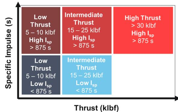
**Fig. 1.** The reactor and engine conceptual design trade space surveyed in this study spanned a wide range of specific impulse and thrust levels.
