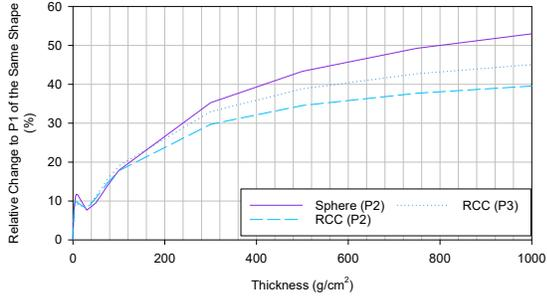
Fig. 4: Relative Change to P1 of the Same Shape as a function of Thickness of Polyethylene
