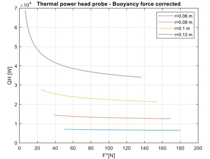
Fig. 2. Probes with different radii are shown considering melting velocity ( $V=0.9$  mm/s) and different values of corrected force. QH is the heat power at the probe head.
