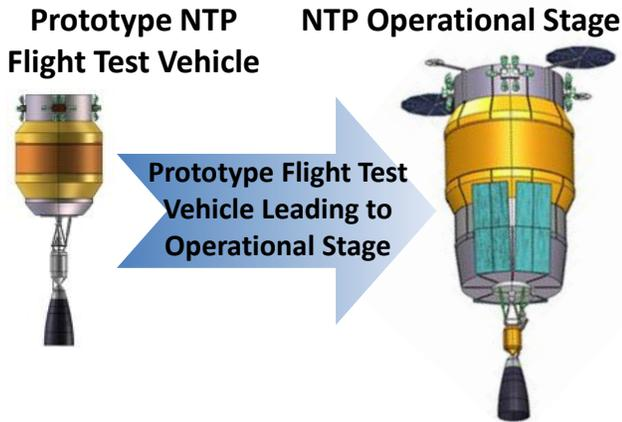
**Fig. 9.** A prototype NTP flight test vehicle can be evolved for use on future operational missions<sup>1</sup>
