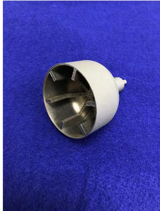
**Fig. 4.** Additively manufactured heat pipe condenser
