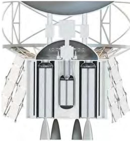
Figure 9: Assembly of subcores in the full core. The central subcore is reduced in size and equipped to provide electrical power.
