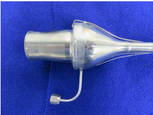
**Fig. 3.** Stirling hot end integrated into heat pipe condenser
