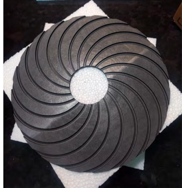
Figure 1: A graphite based SPRINTR fuel plate.
