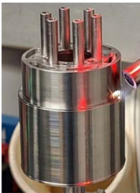
Figure 6 – SRSC magnet can assembly
