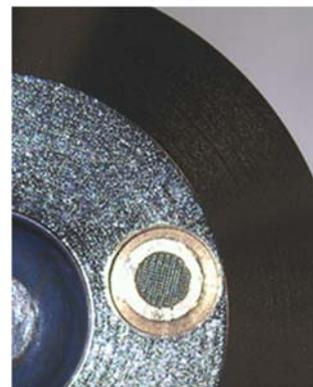
Figure 5 – Gas bearing system entrance filter
