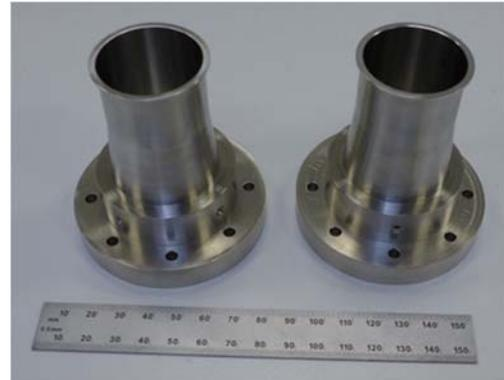
Figure 7 – SRSC heater heads
