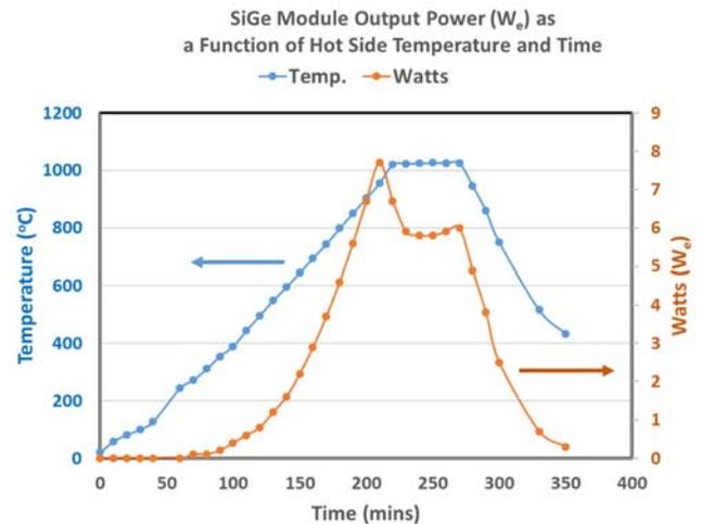
**Fig. 7.** SiGe module output power (W<sub>e</sub>) as a function of hot side temperature and time.
