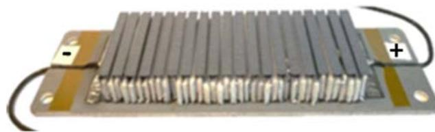
**Fig. 1.** Thermagy™ 20401-13 silicon germanium thermoelectric module obtained from RGS Development BV.<sup>5</sup> Total module dimensions including the substrate are ~4.8 cm by ~16 cm.
