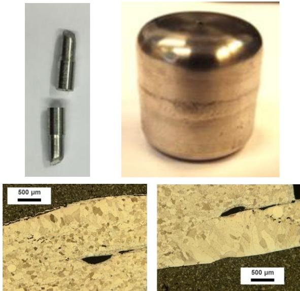
**Fig. 2.** Welding, sectioning and etching of welded structures. The top image on the left shows some small test pieces that were welded and then sectioned and etched. The
