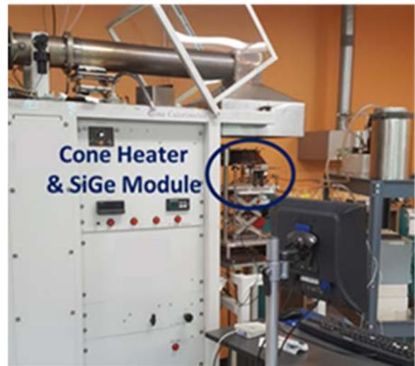
**Fig. 3.** Cone Calorimeter experimental setup showing the location of the cone heater and a SiGe module.
