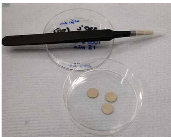
**Fig. 2.** Three porous platinum discs fabricated using the polymeric templating route.
