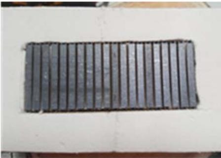
**Fig. 2.** Ceramic insulated SiGe module ready for testing.
