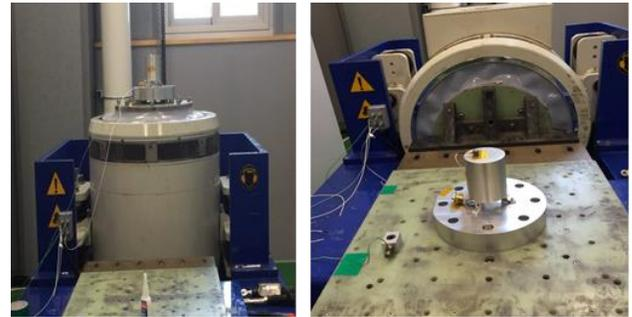
(b) Set up of vibration test
