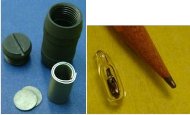
**Fig 4.** Graphite irradiation capsule and cadmium filter (left) and a target contained in a quartz ampule (right).
