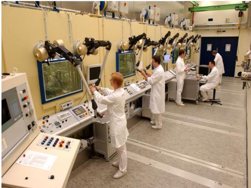
**Fig. 5.** The shielded gloveboxes with installed manipulators for in the minor actinides laboratory at JRC Karlsruhe.<sup>8</sup>
