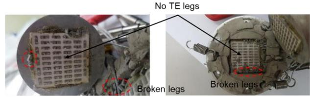
**Fig. 2.** Failure of TE legs after a random vibration test.
